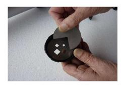
Put the desired disc in the plastic ring,
