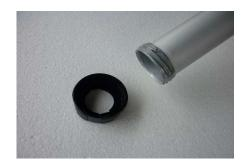
Turn off the lower black plastic ring, fill up cylinder max. to half with not too hard clay
